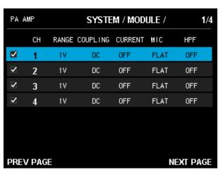
4 Select the channel to set first and press the ENTER button to open the settings screen.
