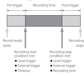
For trigger recording, you can set a combination of recording starting conditions (level trigger, external trigger or timeout) and recording stopping conditions (level trigger, external trigger or recording time).
