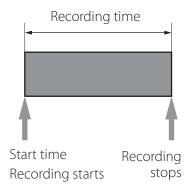
With interval recording, when the Number of repetitions is set to 1, recording will start at the Start time and stop after the set Recording time has elapsed.
