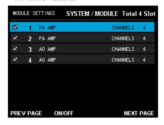
3 Select the module to set first and press the ENTER button to open the settings screen.
