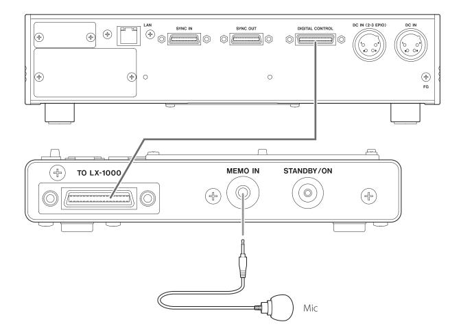
Use the included cable to connect the DIGITAL CONTROL input/output connector on the back of the LX-1000 to the TO LX-1000 control input/output connector on the back of this unit.
