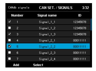
4 After putting checks next to all the signals to load, press the Add (F1) button to add them.
