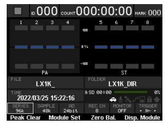
When a submenu screen is open, press the MENU/ HOME button to return to the Menu Screen page above it.
