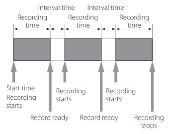
If the number of repetitions is set to 2 or more, recording will start at the Start time and stop after the set Recording time has elapsed. After the Interval time has elapsed, recording will start again, repeating for the set Number of repetitions. Then, recording will stop.
