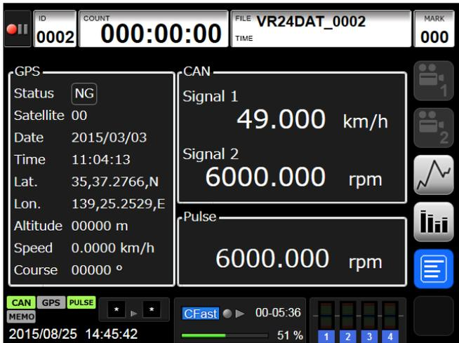
When GPS, CAN or Pulse is active, you can select it. Unused functions are shown as OFF.
