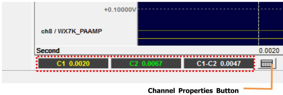
"Channel Properties Button" can be used to open "Channel Properties List" at under the waveform display area.
