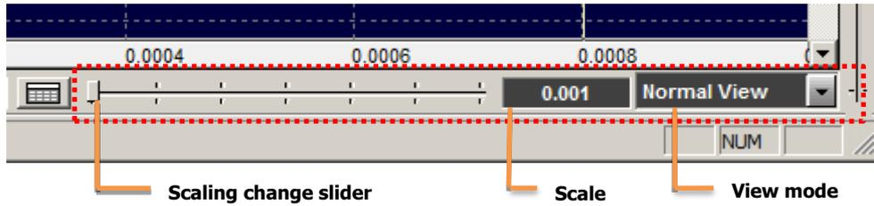
"Scale" is corresponding to the number of seconds from the left to the right of the waveform display area".
