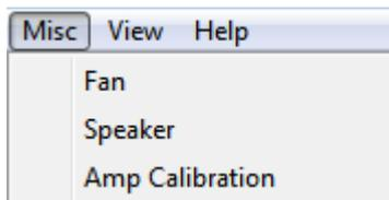
Fan: Stop the fan forcibly for 10 minutes when recording or playback.
