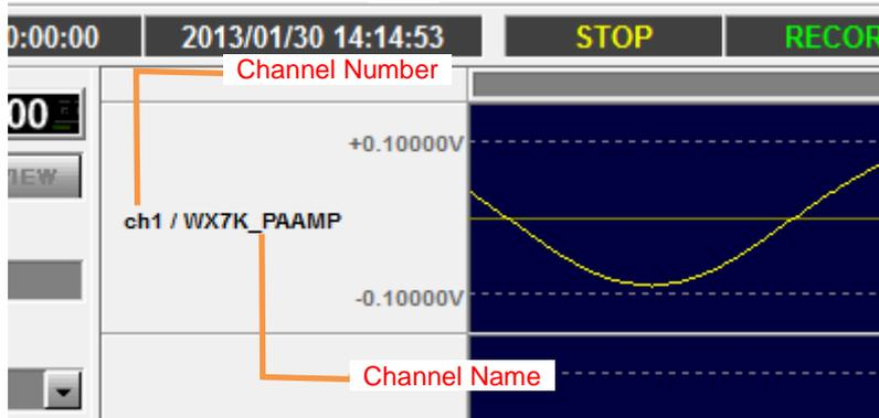
By dragging channel information area, changing display order and overlapping waveform are possible.
