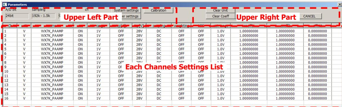
Each channels "Unit", "Channel Name", "Use", "Input Range", "Sensor Current", "Sensor Voltage", "Coupling", "Weighting", "HPF", "Output Range", "Coeff 1", "Coeff 2" and "Offset" are able to change.
