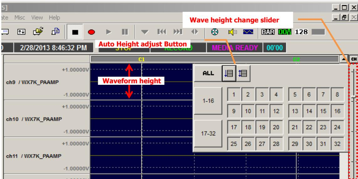
If you'd like to manually adjust the height of the waveform, "Wave height change" slider can be used. All channels will be adjusted at the same height. It is not able to display. It is not possible to change the height for each channel.
