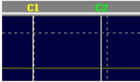
The left edge is 0[sec] and the right edge is defined seconds by "scale" in the waveform display area, time positions of the "C2" and "C1" cursor are displayed. "C1-C2" is the time differences between 2 cursors.
