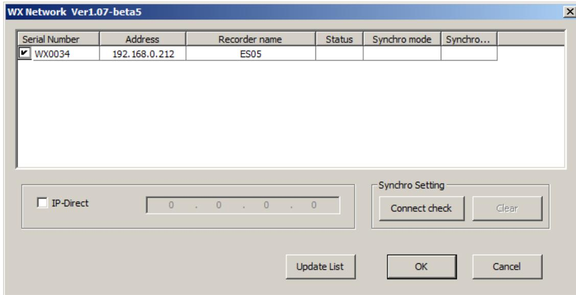
Check the box at the serial field WX Network dialog box by confirming that the white-out box has appeared and the correct serial number are displayed, and then click OK. In addition, a previously used serial number will automatically contain a check in the box.
