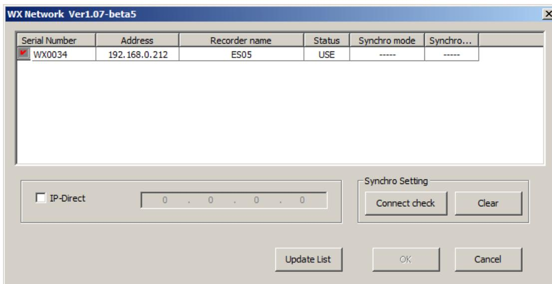
If a TCP connection is not possible because of a problem such as an incorrect IP address for the same segment, a grey check box will be displayed along with IP ERR in the status field. In that case, specify an appropriate IP address or check the IP address settings (Subnet mask, Gateway, etc.) between the PC and the WX-7000, and then connect to the WX-7000 series.
