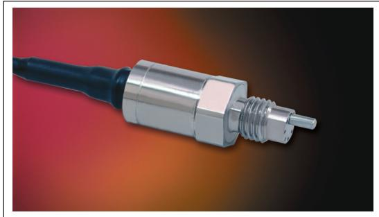
The ETL/T-312 is a miniature threaded pressure transducer/platinum RTD combination. The pressure transducer utilizes a patented silicon on silicon design. The platinum RTD protrudes beside the diaphragm to sense media temperature. The pressure and temperature devices are designed to operate independently. All wetted parts of the transducer are compatible with most automotive fluids.
