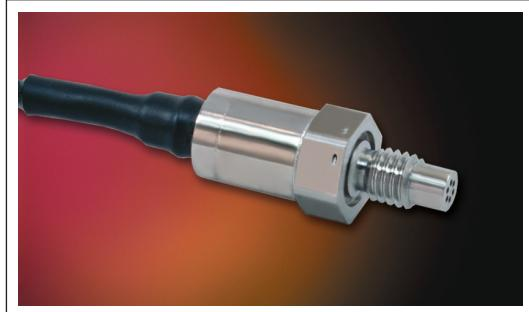
The MAKS-6(X) is one of the newest generation of Kulite's smallest miniature amplified transducers currently available. The sensing sub-assembly is protected from mechanical damage by a protective screen, which has been shown to have minimal influence on the frequency response of the sensor.
