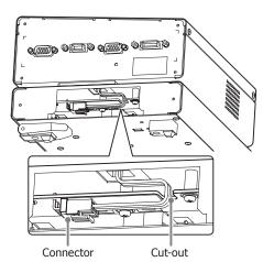
• Wire the connection cable through above cut-out
